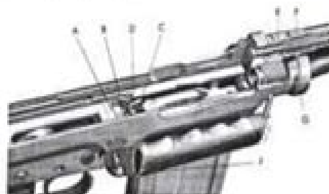
Figure 1 - Detail of Rifle Locking Mechanism
